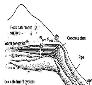
**Rock catchment** systems retain rainwater and channel it through pipelines into big solid basins. The run-off rain water will be retained and piped into water basins. Costs for such a system will be about 80.000 Euros. This will provide about 3.000 people in this region with drinking water.
